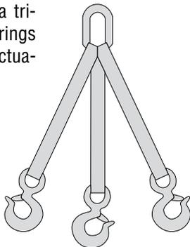
Figure 5: Triple-leg sling
