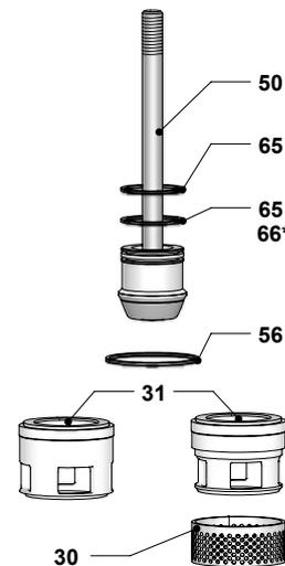
Figure 13: Extended bonnet trim for pressure balanced designs
