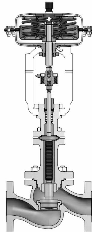
Figure 2: Valtek GS with Bellows Seal Bonnet
