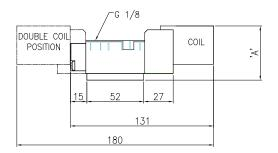
The coil itself can be rotated in 90° steps by releasing the four securing screws. (FIG 3) When rotating the coil care should be taken to ensure the core assembly (core, spring, seal and washer) remains intact and alined correctly. This is easily achieved by only lifting the coil the small amount required to clear the screws enabling the coil to be rotated.
