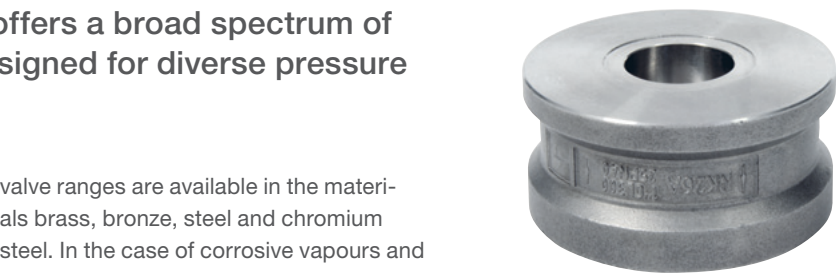
RK 26A with self-centering body, PN 10 to 40, DN 15 to 100 (1/2 to 4"). Facings suitable for counterflanges to ASME 150 RF, ASME 300 RF, tongue or male flanges to DIN EN 1092. Material: austenitic steel
