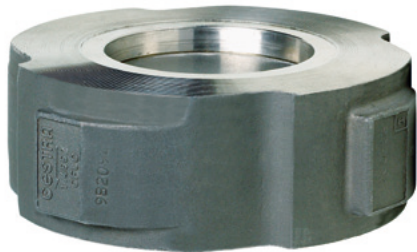
RK 86 und 86A with patented universal centering. As standard unit, it fits between flanges for PN 6–40, Class 150/300 and also between BS10 flanges. Body material: stainless (RK 86) or austenitic steel (RK 86A). Valve disc: austenitic steel
