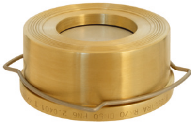
RK 70 with spiral centering PN 6, body material hot-pressed brass, valve disc of PPO
