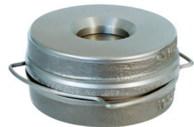
RK 49 with spiral centering, for high temperatures, PN 63/100/160, DN 15 to 200 (1/2 to 4"). Material: high-temperature austenitic cast steel/high-temperature cast steel
