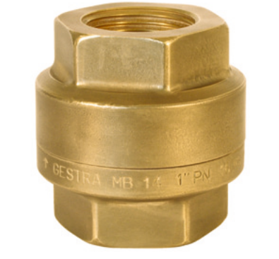
MB 14 Screwed 1/2–2" BSP, body material hot-pressed brass, valve disc of austenitic steel
